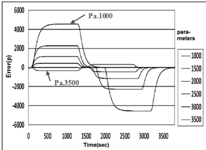
Fig. 8. Waveform showing the synchronization error with parameters 4065~4068
