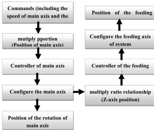
Fig. 1. Control architecture of rigid tapping
