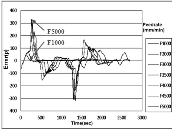
Fig. 7. Waveform showing the synchronization error under original parameters
