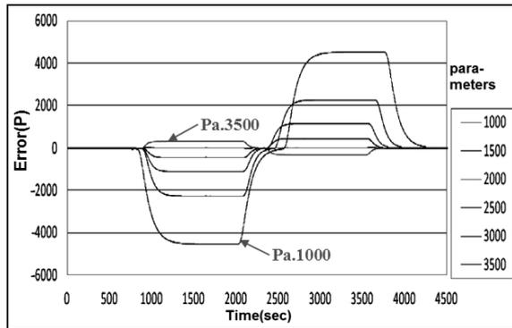
Fig. 9. Waveform showing the synchronization error with parameters 5280~5283
