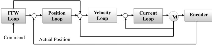
Fig. 3. Feed-forward integrated  $Z$  axis servo controller
