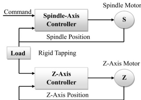
Fig. 2. Synchronous control system
