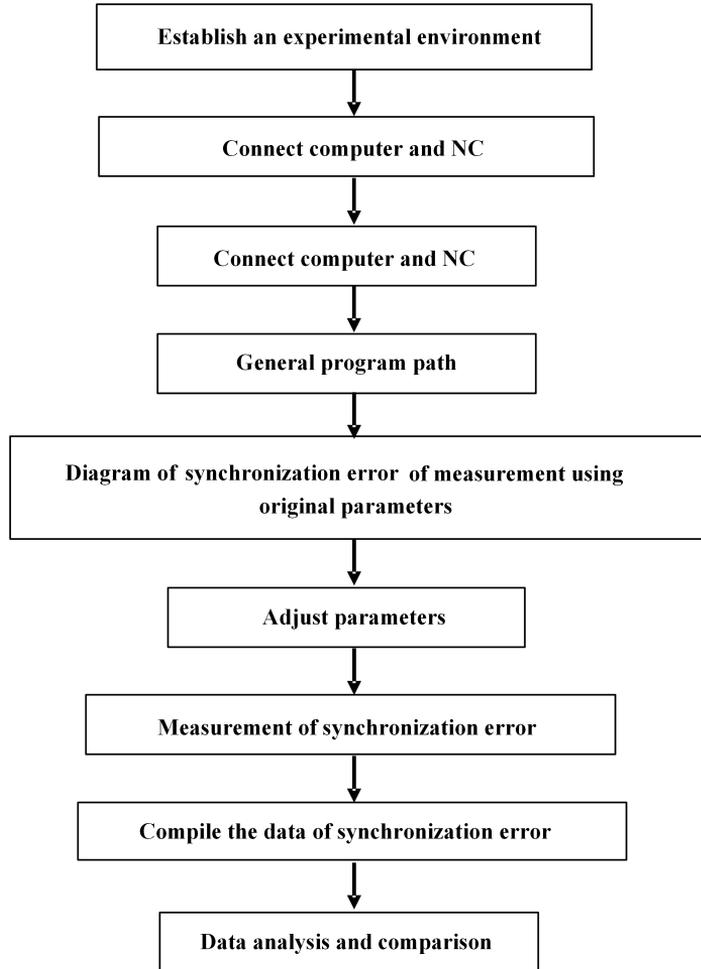
Fig. 5. Flowchart of experiment
